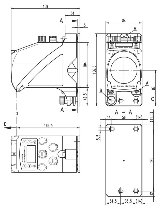
A M5 screw for alignment
