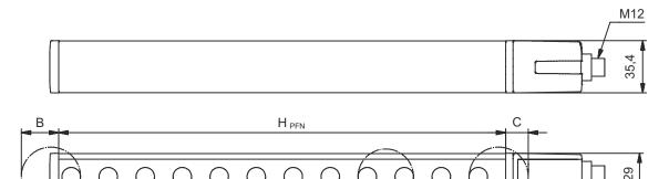
$H_{\rm PFE}$  Effective protective field height = 2490 mm  $H_{\rm PFN}$  Nominal protective field height = 2400 mm
