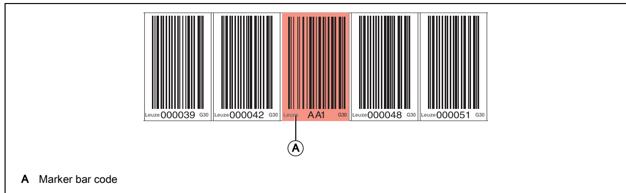
Figure 5.5: System arrangement of marker bar code
