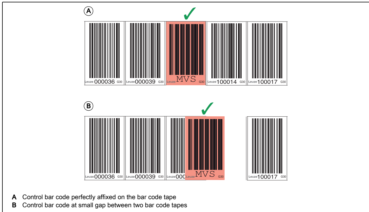
Figure 5.3: Correct positioning of the control bar code
