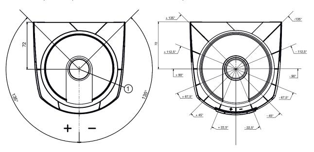
Reference point for distance measurement and protective field radius
