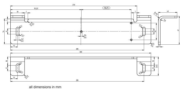
Fig. 14.3: Mounting bracket BT-MSI-MD\_FB-L
