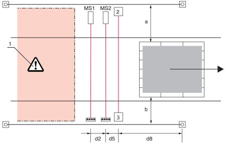
1 Danger zone 2 Muting transceiver 3 Passive deflecting mirror MS1 Muting sensor 1 MS2 Muting sensor 2 Distance between pallet and hard quard a, b Distance between MS1 and MS2 d2 d5 Distance from the light-beam of MS2 vertically to the protective-field plane Distance from the end of the mechanical protective device, e.g. a hard guard, to the protective d8
