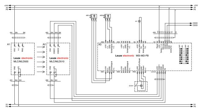
Fig. 7.3: Circuit diagram example: timing controlled 2-sensor muting
