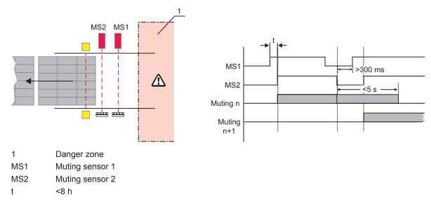
Fig. 4.4: Muting for tight sequences of objects – arrangement of the muting sensors and timing
