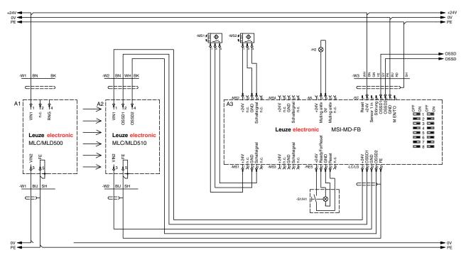
Fig. 7.4: Circuit diagram example: sequence controlled 2-sensor muting
