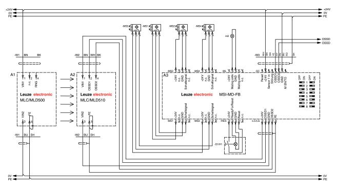
Fig. 7.5: Circuit diagram example: sequence controlled 4-sensor muting
