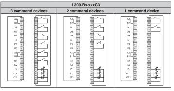
4.10.4 Switch with integrated command devices and M23 connector, 19-pin
