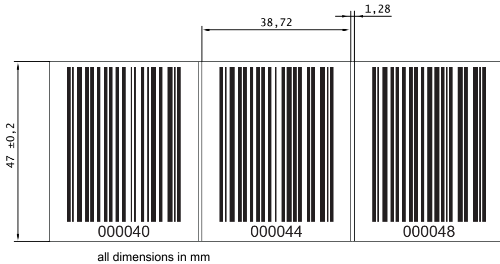
Figure 13.10: Dimensioned drawing bar code tape BCB with 40 mm grid
