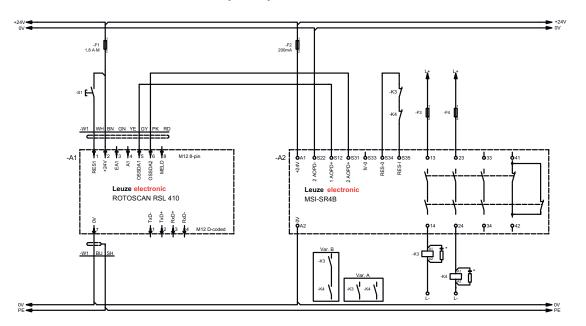
Spark extinction circuit, suitable spark extinction provided
