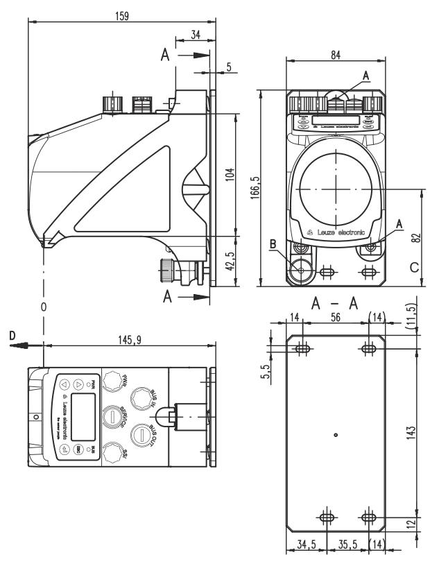
A M5 screw for alignment
