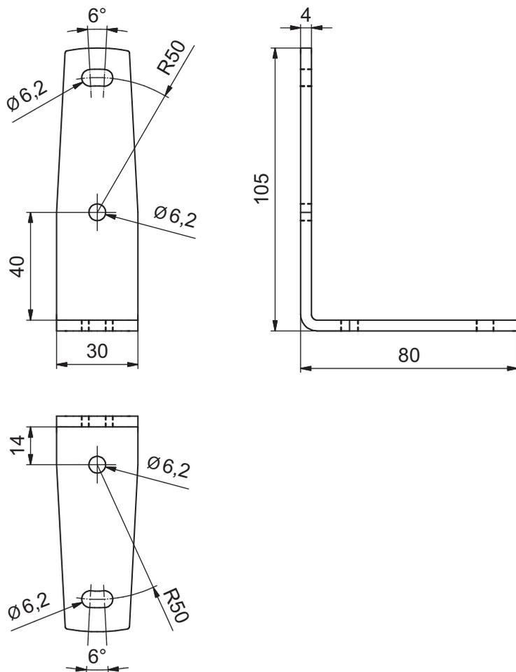
Fig. 14.8: Connection bracket for L-shape or U-shape
