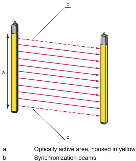
Fig. 3.1: Transmitter-receiver system
