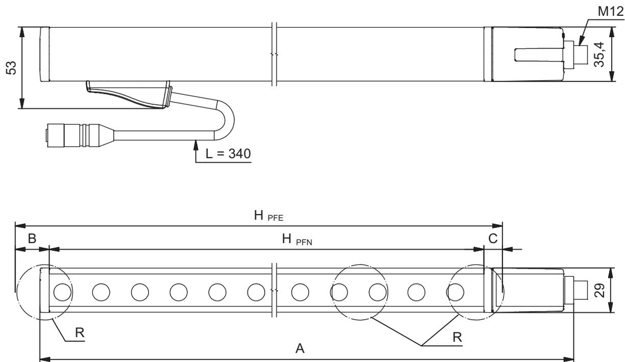
Fig. 14.1: Dimensions of Host transmitter and Host receiver
