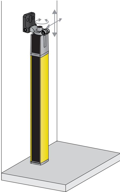
Fig. 6.10: Mounting directly on the machine table
