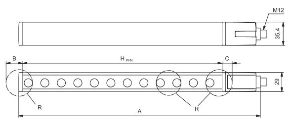
$H_{\mathsf{PFE}}$  Effective protective field height = 340 mm  ${\rm H_{PFN}}$  Nominal protective field height = 300 mm
