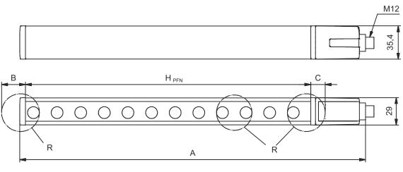
$H_{\mathsf{PFE}}$  Effective protective field height = 612 mm  $H_{\mathrm{PFN}}$  Nominal protective field height = 600 mm
