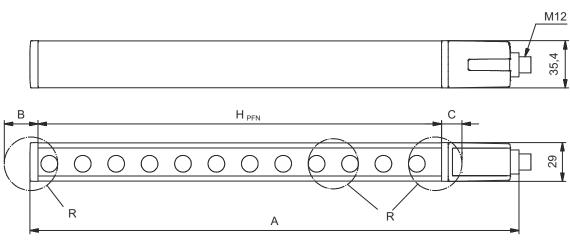
$H_{\mathsf{PFE}}$  Effective protective field height = 1390 mm  $H_{\mathrm{PFN}}$  Nominal protective field height = 1350 mm
