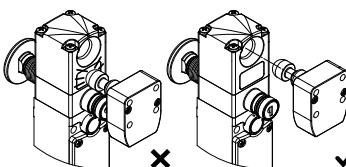
**⚠️** Attention: Although the device is designed to facilitate alignment between the device and actuator, excessive misalignment could damage the device. Periodically check the correct alignment between the safety device and its actuator.
