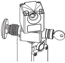
Before mounting the device: if necessary, it is possible to adjust the position of the head and the auxiliary release (if present) in order to turn the device to the most appropriate position for the specific application. Fully remove the 4 head screws in order to independently turn either the head or the auxiliary release over an arc of 270°.
