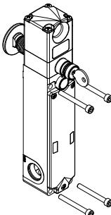
**⚠️** Attention: Always fix the device with 4 M5 screws with property class 8.8 or higher, and flat seating heads. Install the screws with medium thread lock, and a number of threads engaged equal to or greater than the screw diameter. The device must never be fixed with less than 4 screws. Tighten the 4 M5 screws to a torque from 2 to 3 Nm.
