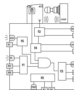
In the initial "POWER ON" status, function f0 of the safety device carries out an internal self-diagnosis which, if successfully completed, brings the device to the "RUN" operating state. If the test is not passed due to an internal fault, the device enters the "ERROR" status.
