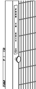
For installation on walls thicker than 20 mm, extensions are available for the release button.
