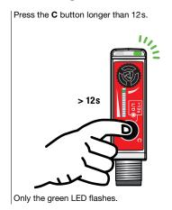
Release the button. LED on = >12s PNP light switching, **OUT1** (Pin 4): NPN dark switching OUT2 (Pin 2) 1): PNP dark switching, NPN light switching LED off = >12s **OUT1** (Pin 4): PNP dark switching, /D ( NPN light switching OUT2 (Pin 2) 1): PNP light switching, NPN dark switching 1) Only for devices without analog output
