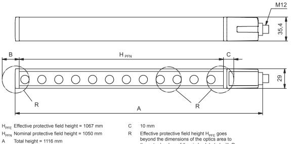
В 7 mm Effective protective field height H<sub>PFE</sub> goes beyond the dimensions of the optics area to the outer borders of the circles labeled with R.
