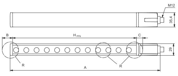
$H_{\mathsf{PFE}}$  Effective protective field height = 762 mm  $H_{\mathrm{PFN}}$  Nominal protective field height = 750 mm
