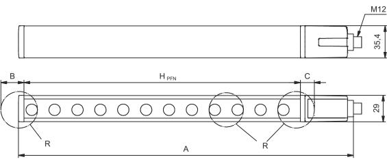
$H_{\rm PFE}$  Effective protective field height = 628 mm  $H_{\rm PFN}$  Nominal protective field height = 600 mm
