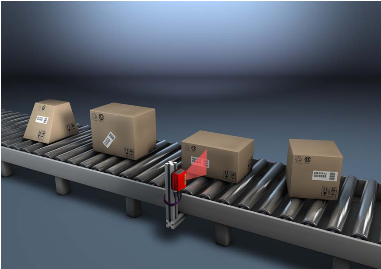
Figure 4.1: Possible bar code orientation
