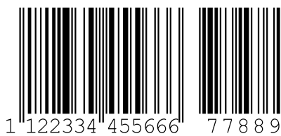
Figure 18.6: Code type 10: EAN 13 Add-on
