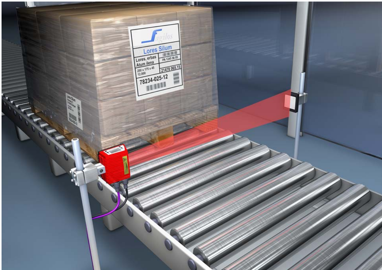
Figure 4.2: Reflector arrangement for autoReflAct
