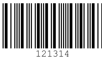
Figure 18.15: Code type 11: Codabar
