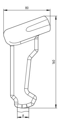
A Cable entry: depending on the cable, max. Ø 20mm, cable-Ø 5mm
