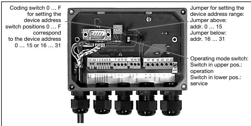
Figure 7.1: Configuration elements in the MA 2
