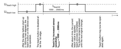
After the teaching, the sensor switches when about 18% of the light beam are covered by the object.
