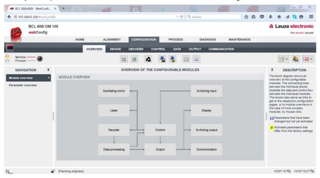
Figure 9.2: Module overview in the webConfig tool
