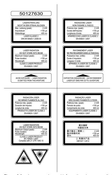
Figure 2.3: Laser warning and information signs – supplied stick-on labels
