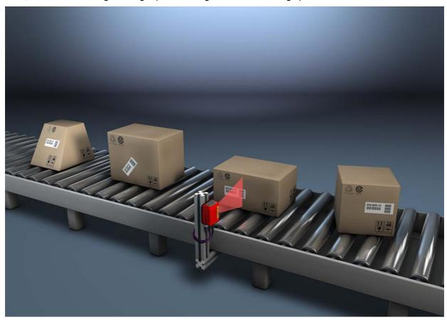
Figure 4.1: Possible bar code orientation
