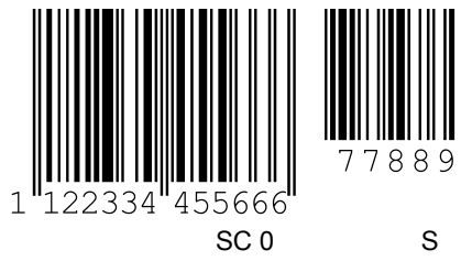
Figure 15.8: Code type 10: EAN 13 Add-on
