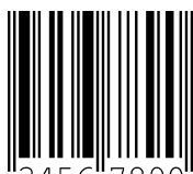
Figure 15.6: Code type 06: UPC-A
