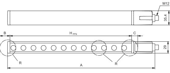
$H_{\mathrm{PFE}}$  Effective protective field height = 928 mm  $H_{\mathrm{PFN}}$  Nominal protective field height = 900 mm
