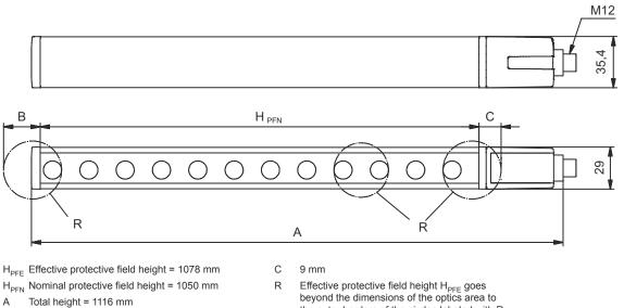
В 19 mm Effective protective field height H<sub>PFE</sub> goes beyond the dimensions of the optics area to the outer borders of the circles labeled with R.
