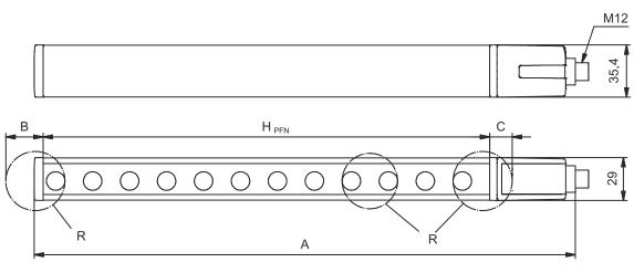
$H_{\mathsf{PFE}}$  Effective protective field height = 2590 mm  ${\rm H}_{\rm PFN}$  Nominal protective field height = 2550 mm
