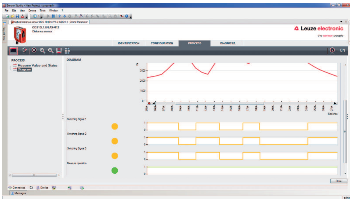
Fig. 8.11: PROCESS function – display of the measurement values
