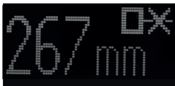
Fig. 8.6: Display: Measurement value frozen in the case of deactivation
