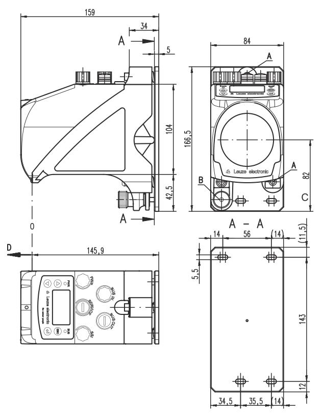
A M5 screw for alignment
