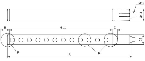
$H_{\mathsf{PFE}}$  Effective protective field height = 478 mm  $H_{PFN}$  Nominal protective field height = 450 mm
