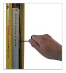
2 Activate the <u>laser beams</u> if necessary by placing the MagnetKey on the transmitter below the red laser exit window.
