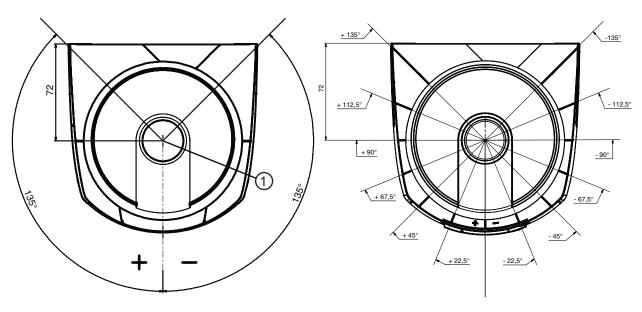
1 Reference point for distance measurement and protective field radius
