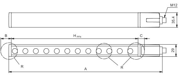
$H_{\text{PFE}}$  Effective protective field height = 1678 mm  $H_{\text{PFN}}$  Nominal protective field height = 1650 mm
