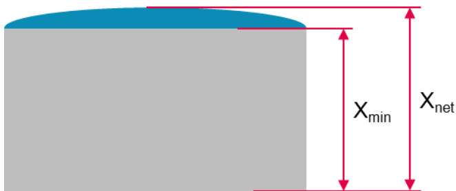
Figure 10: Top view of an object with lateral bulge
