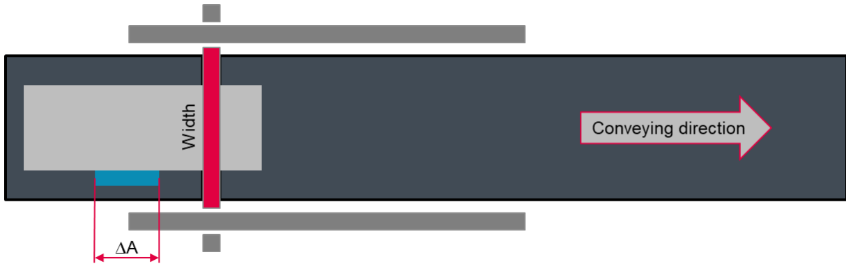
Figure 8: Sketch of an overhang of an object in width direction
