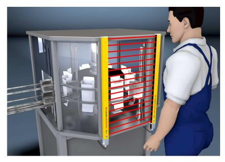
Fig. 5.1: Point of operation guarding protects reaching into the danger zone, e.g. for cartoners or filling systems
