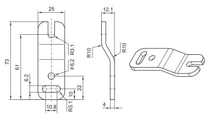
Fig. 14.3: BT-Z parallel bracket
