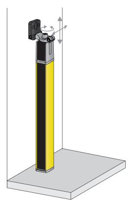
Fig. 6.10: Mounting directly on the machine table
