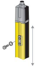
Fig. 6.7: Mounting via sliding blocks BT-NC60
