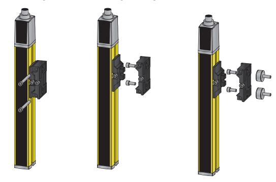
Fig. 6.9: Mounting via swiveling mounting brackets BT-2SB10
