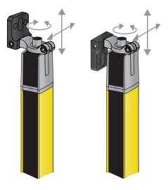
Fig. 6.8: Mounting via swivel mount BT-2HF
