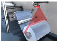
Determining width and diameter of roll goods
