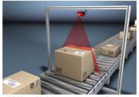
Width and height measurement of cartons
