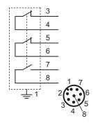
Figure 6.5: Pin assignment of the 8-pin M12 connector (S200-xxx-M12-xxx)
