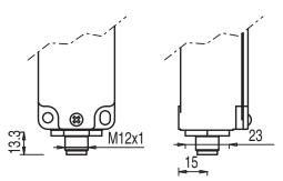
Figure 3.3: Dimensions of S200-M4C1-M12 in mm (here, M12 connector dimensions)
