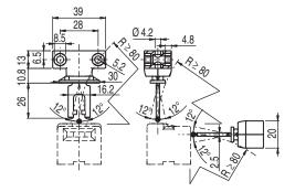
Figure 12.6: AC-AH-F4J2-TK actuator
