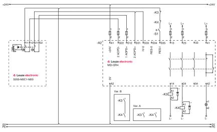
Spark extinction circuit, suitable spark extinction provided
