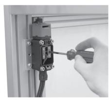
♥ Tighten the housing cover with 0.8–1.2Nm.
