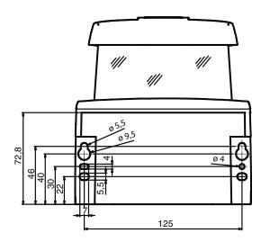
Minimum space requirements for installation and replacement of scanner unit
