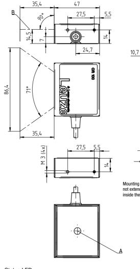
Mounting screws M3 should not extend more than **3mm** inside the housing!
