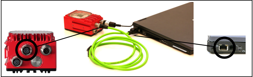
Figure 6.1: Connecting the LSIS 4xx i to the PC
