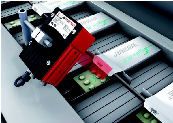
Figure 3.4: Application example: code verification
