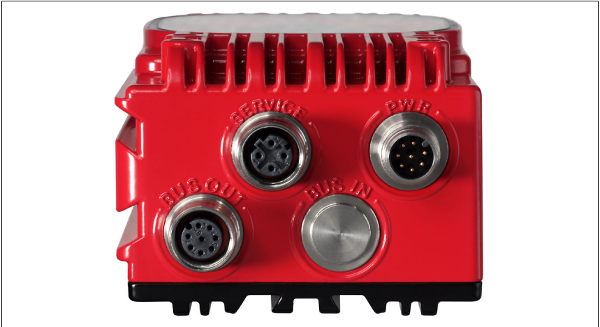
Figure 5.1: Location of the electrical connections
