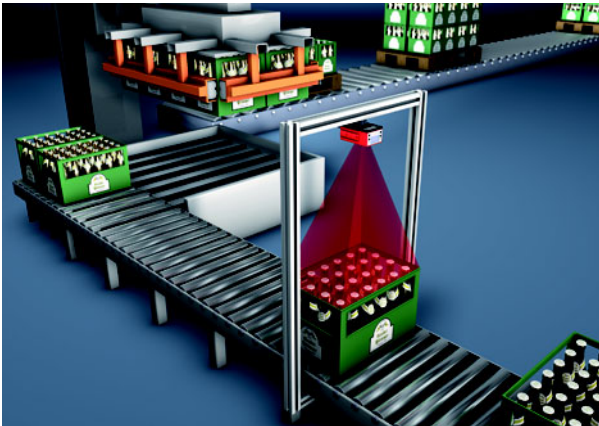
Figure 3.2: Application example: completeness monitoring
