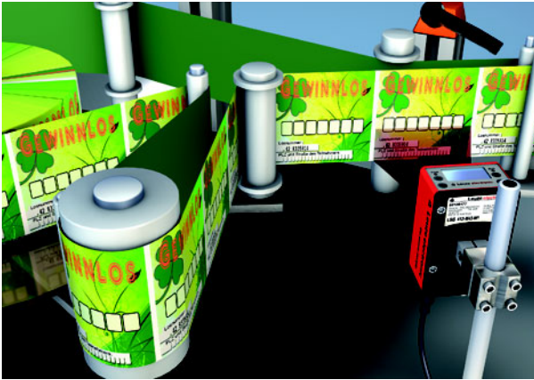
Figure 3.1: Application example: presence monitoring
