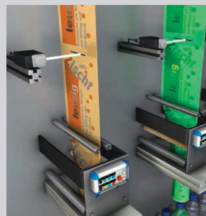
Reliable mark detection when cutting sleeve labels
