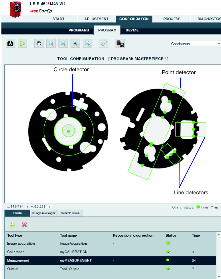
Figure 3.34: Detectors of the measuring tool in the camera image display
