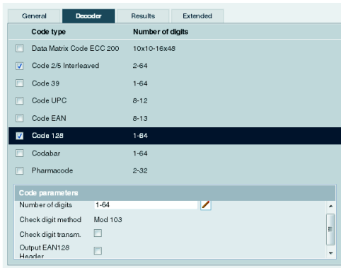
Figure 3.28: Decoder parameters of the code tool
